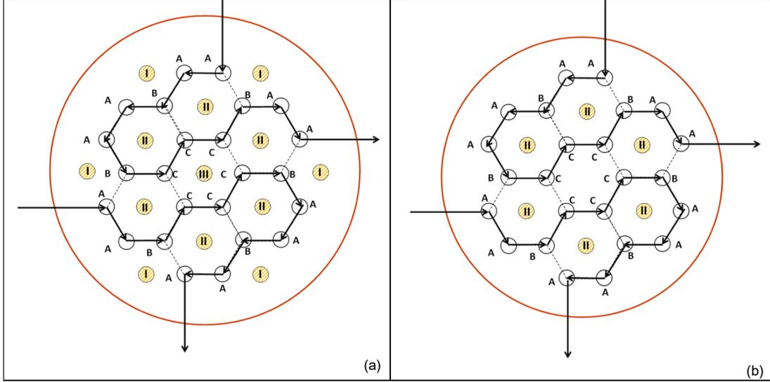
Figure 3: Arrangement of heating elements (locations I, II, and III) and tubes (locations A, B, and C) in the furnace; a) scheme 1; b) scheme 3.
