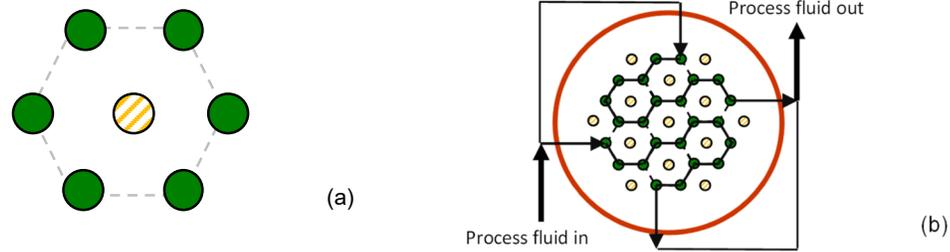
Figure 2: a) Basic “hive” cell: Tubothal® heating elements: yellow; process fluid tubes: green; b) Arrangement of heating elements, process fluid tubes and fluid passes.
